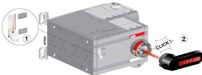
Figure 3.3 Operating the motorized switch-disconnector manually
