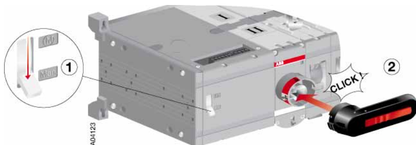
Figure 3.3 Operating the motorized change-over switch manually
