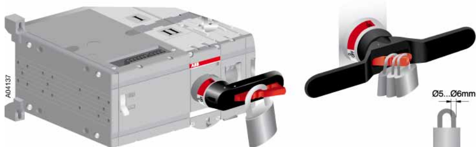
Figure 3.4 Locking the manual operation
