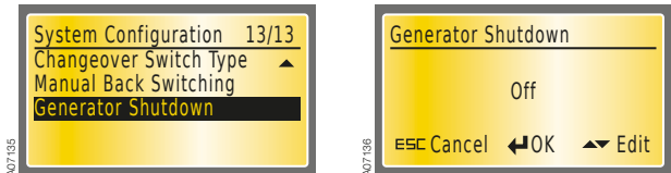
Figure 7.22 Generator Shutdown, Off is the default
