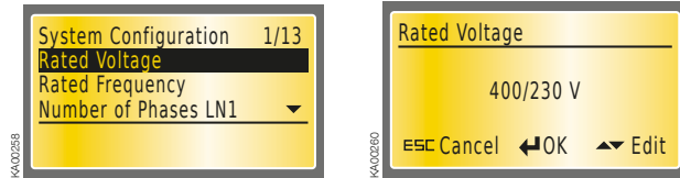
Figure 7.10 Rated Voltage, factory setting is 400/230 V
