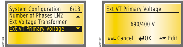
Figure 7.15 Ext VT Primary Voltage, factory setting is 690/400V
