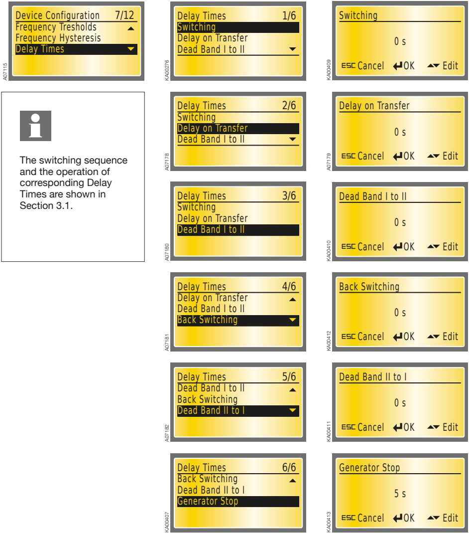
Figure 7.40 Switching 0 s, Delay on Transfer 0 s, Dead Band I to II 0 s, Back Switching 0 s, Dead Band II to I 0 s, Generator Stop 5 s
