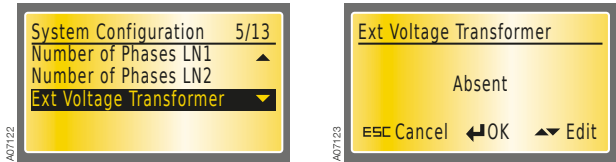
Figure 7.14 Ext Voltage Transformer, Absent is the default
