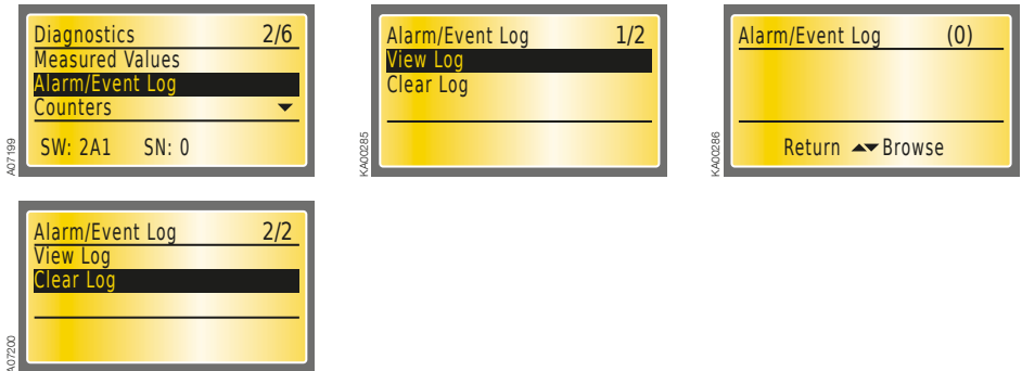
Figure 7.49 Alarm/Event Log: View Log will show 50 latest alarms and events, Clear Log will empty the log
