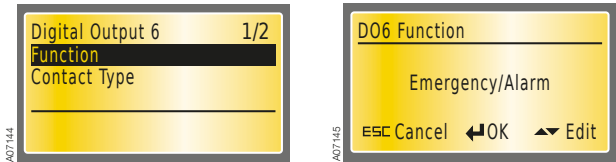
Figure 7.28 Digital Output 6 - Function, Emergency/Alarm is the default
